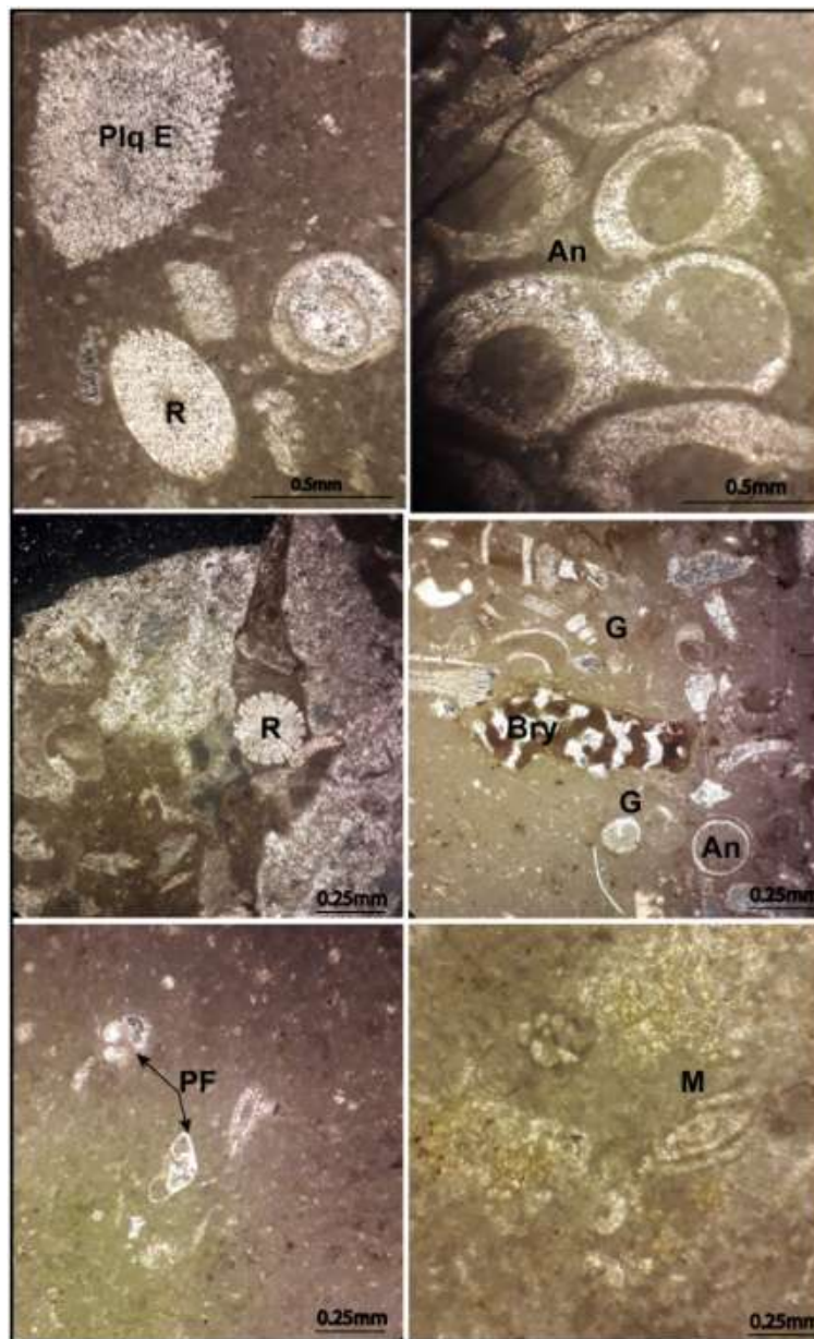
Figure II. 8: Wackestone to packstone limestone with large fragments of invertebrates and miliolae (M) rare planktonic foraminifera (PF) and bryozoans (Bry).
