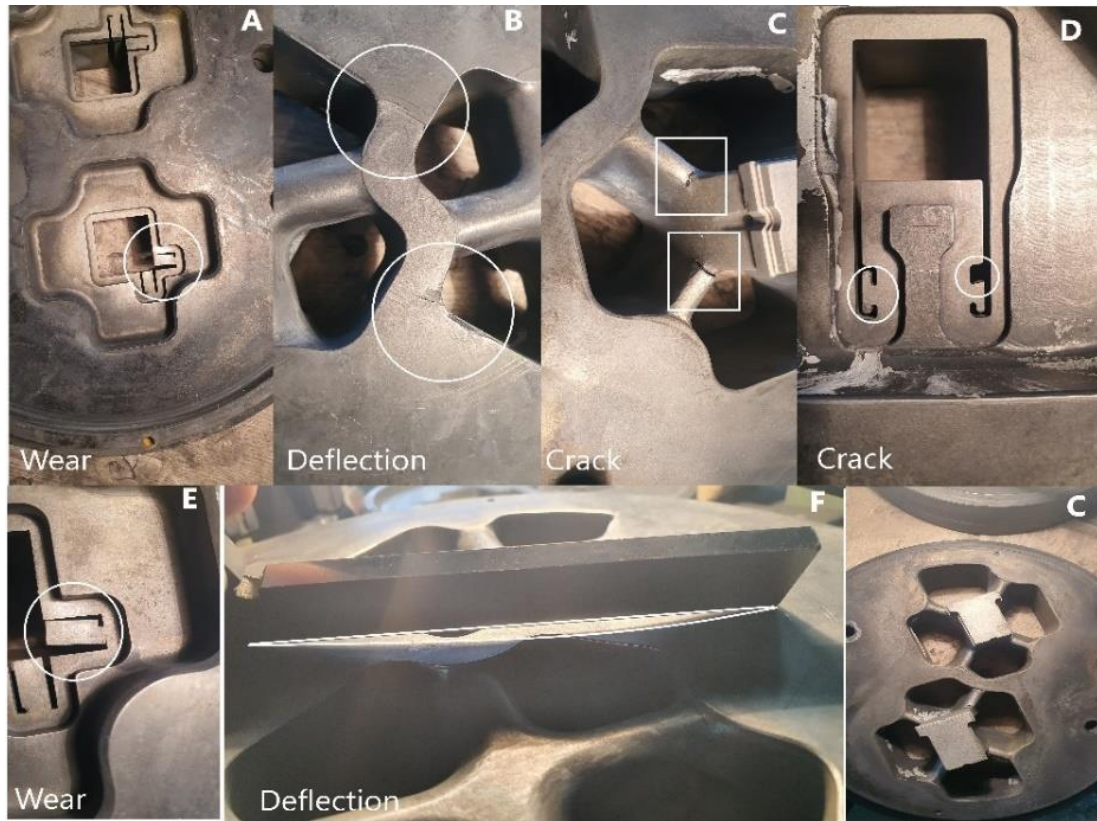
Figure III.29: The most important failures of aluminum extrusion dies
