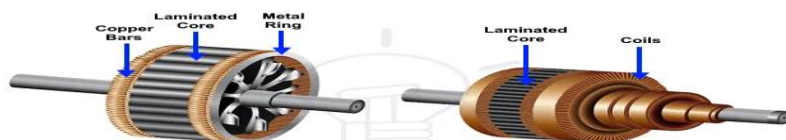
Figure 1.3: Squirrel cage rotor (left) and wound rotor (right)
