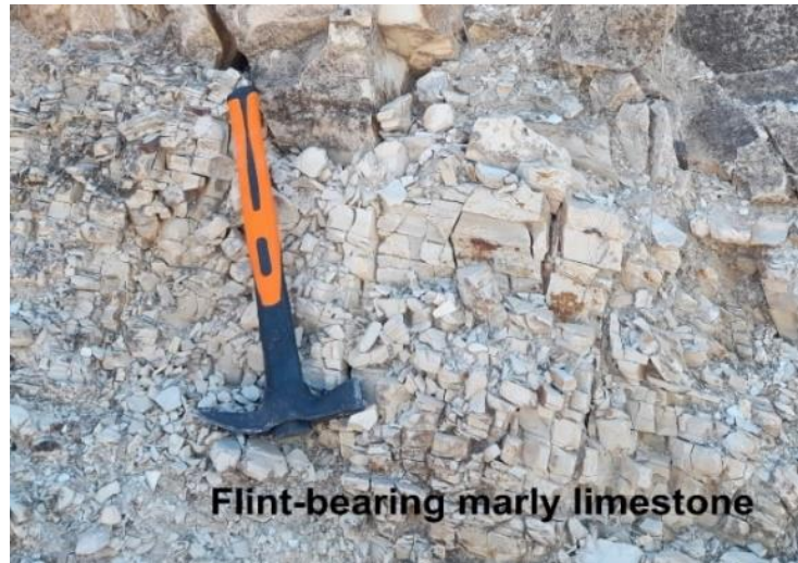
Fig. II. 44. Field photograph showing beige, semi-friable, flint-bearing marly limestone of Ain Kissa deposit.
