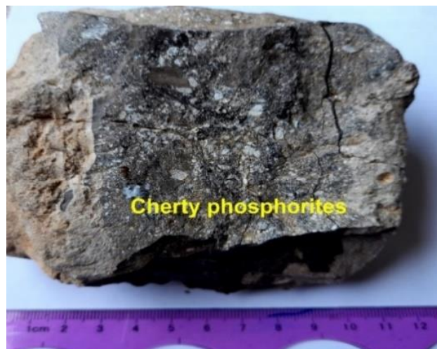
Fig. II. 9. Hand specimen showing hard, grey cherty phosphorite with abundant phosphatic particles from Troubia deposit.
