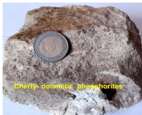
Fig. II. 11. Hand specimen showing hard, grey dolomitic-cherty phosphorites with abundant medium to coarse-grained phosphatic particles from Troubia deposit.
