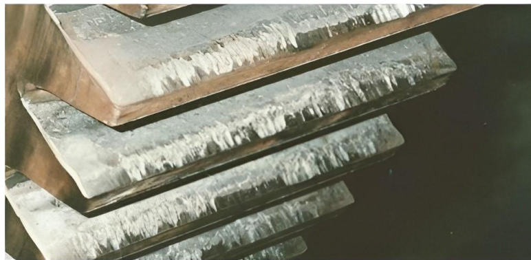
Figure 2.23 Real gear seizure fault [103].
