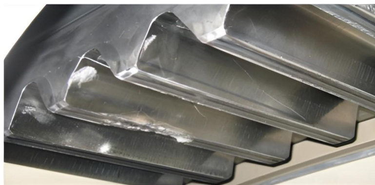
Figure 2.24 Real gear crack defects [103].
