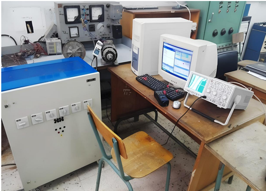
Figure 4.1 Test Bench Configuration for Simulating Mechanical Faults in Induction Motors.
