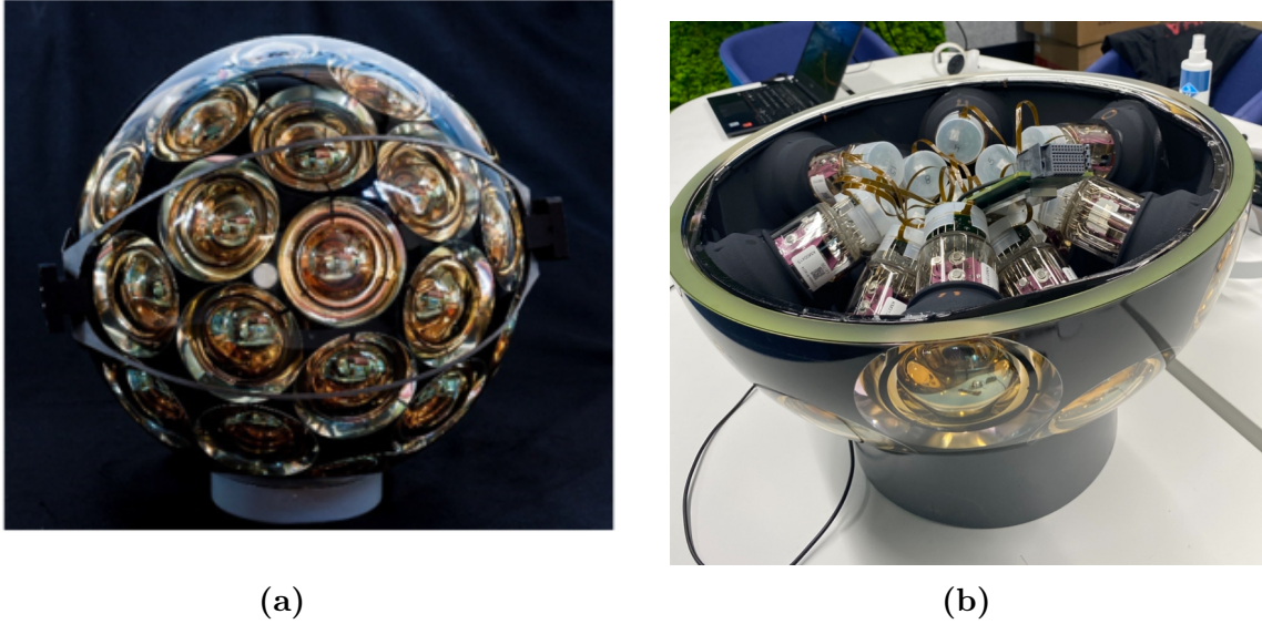
Fig. 3.5: KM3NeT digital optical module. (a) fully assembled DOM. (b) DOM with the upper hemisphere removed showing the internal arrangement of PMTs. Taken from [3].
