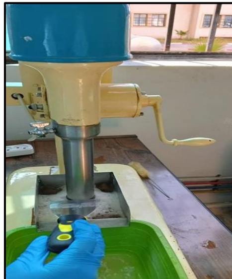
Figure 5.2. Cellule de flottation.
